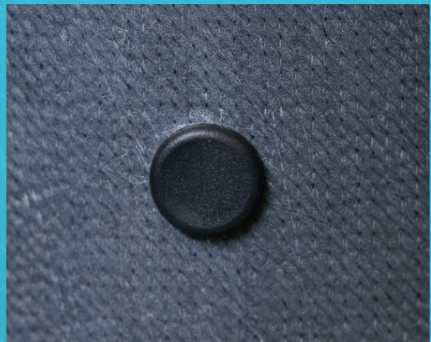
FIG. 10.2 Hole plug installed
