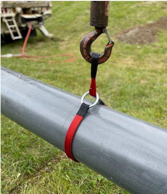
FIG 9.1 Rubber belt grip sling
